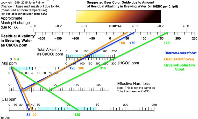
1. Draw a line between the Calcium and Magnesium concentrations to determine the Effective Hardness of your water.
